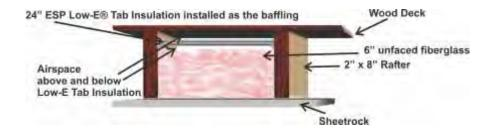
SYSTEM R-VALUES FOR ESP LOW-E® INSULATION AS PER ASTM C-976, AIR TO AIR, ADJUSTED TO MEET CRITERIA EQUIVALENT TO ASTM 1224
