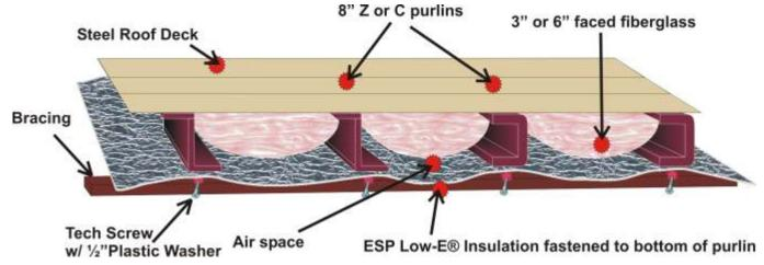
SYSTEM R-VALUES FOR ESP LOW-E® INSULATION AS PER ASTM C-976, AIR TO AIR, ADJUSTED TO MEET CRITERIA EQUIVALENT TO ASTM 1224
