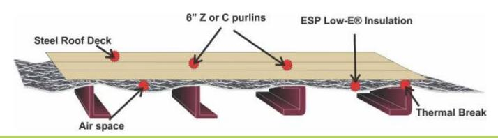
Average System R-Value: Down R- 21.04 (3" Fiberglass), Down R- 30.04 (6" Fiberglass) Up R- 17.38 (3" Fiberglass), Up R- 26.39 (6" Fiberglass)
