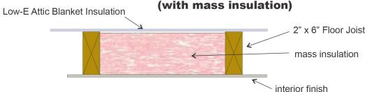
Low-E Attic Blanket can be rolled out over existing mass insulation. The product is perforated and will not trap moisture. Low-E Attic Blanket can be stapled with 1/2" staples every 6". Since it is not a vapor barrier taping of seams is optional.
