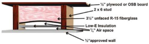
THE SYSTEM R-VALUES FOR THESE INSTALLATION METHODS WERE CALCULATED USING DATA FROM THE 1989 ASHRAE HANDBOOK OF FUNDAMENTALS.
